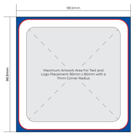
Artboard Size should be set to 98.5mm x 98.5mm with a corner radius of 9mm. Background Images and/or Colours should extend to this dimension.
